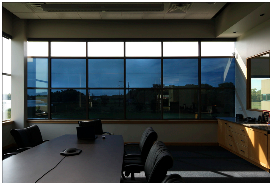
Figure 4. Conference room with zoned SageGlass windows block the sun's glare but allow in sufficient daylight to illuminate the room without the use of artificial lights.
