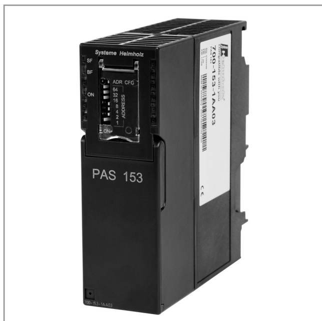
PAS 153, distributed PROFIBUS Interface
