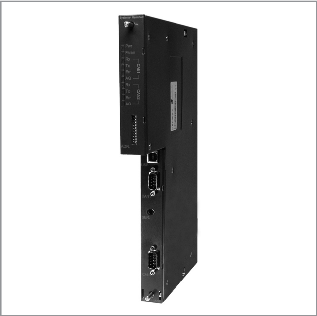
CAN 400, communication module
