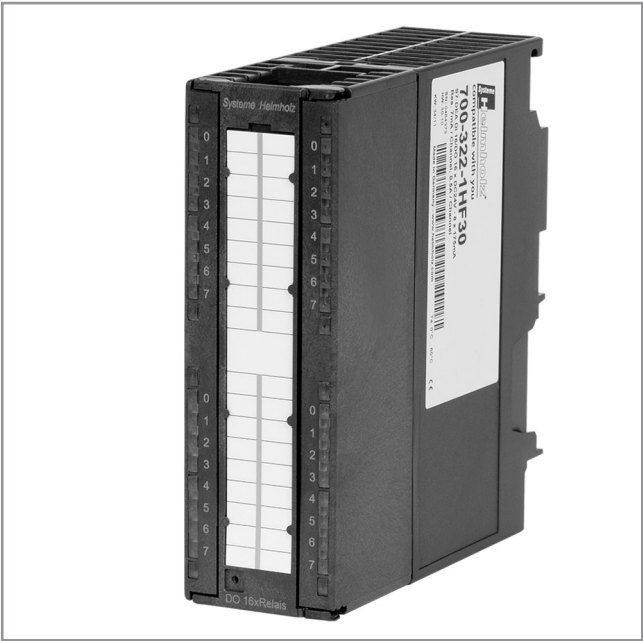
DEA 300, Digital Output; Relays Bistable
